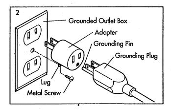
The temporary adapter should be used only until a properly grounded outlet (Drawing 1) can be installed by a qualified electrician. The green-colored ear, lug, or the like extending from the adapter must be connected to a permanent ground such as a properly grounded outlet box cover. Whenever the adapter is used, it must be held in place by a metal screw.
